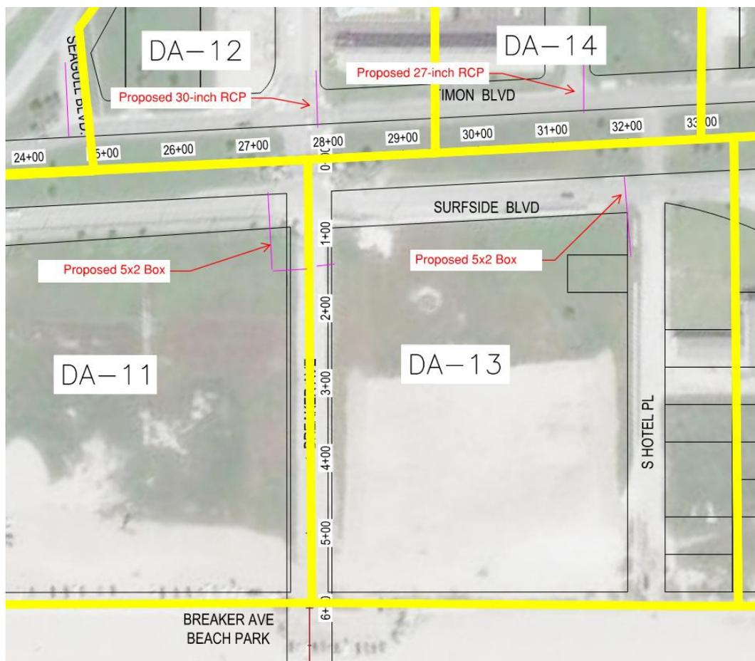
Figure 4-2 – Snapshot of DA's 11-14 – connections to Navigable Canal
