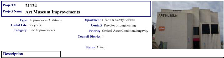
This scope will replace seven of the ten skylights at the Johnson & Burgee Building. The remaining three skylights have not experienced water leaks and do not require replacement at this time. The project will provide the Legorreta building with new storefronts at the main entry, café, and between the small gallery and the exterior water feature. The café will acquire new windows in the dining area overseeing the Harbor Bridge and the Texas State Aquarium.
