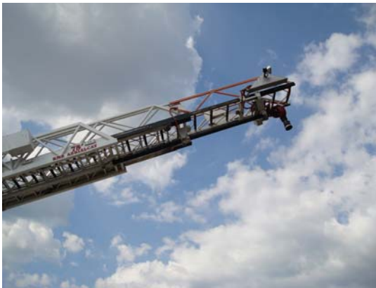
Photo 2 – Aerial ladder with monitor at tip
